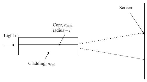
d) In an experiment, light is transmitted along the glass fibre before leaving at a perfectly vertical end. A screen is placed a long distance away from the end of the fibre and a uniform circular spot is seen as shown above. A small glass tank containing water is placed in front of the beam so it perfectly touches the end of the fibre. You may assume the tank is parallel to the screen. On a copy of the above diagram, sketch how the extent of the spot on the screen changes. [2]
