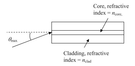
Light may only be transmitted along the fibre if the incident angle of the light is less than a maximum angle  $\theta_{\text{max}}$ . By using your expression from part b) and Snell's law, or otherwise, derive an expression for  $\theta_{\text{max}}$  in terms of the core and cladding refractive indices only. [3]
