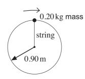
At the top point of the circle the speed of the mass is  $8.2\,\mathrm{m\,s^{-1}}$ . What is the tension in the string at this point?
