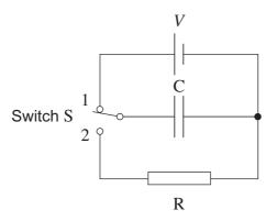
The switch is then moved quickly to position 2, allowing C to discharge through the fixed resistor R. It takes  $36\,\mathrm{ms}$  for the pd across C to fall to  $\frac{V}{2}$ . What period of time must elapse, after the switch has moved to position 2, before the energy stored by C has fallen to  $\frac{E}{16}$ ?
