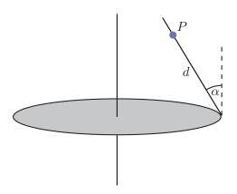
By considering moments about the hinge for the (light) rod, show that the force exerted on the rod by P is parallel to the rod.
